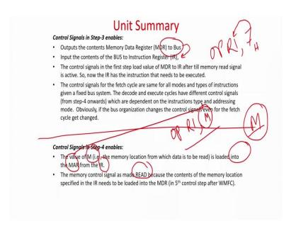
In step 3, basically the memory tells that it is ready and the memory data register now has the instruction which is now loaded because the memory is ready then actually this memory data register transfers the instruction to the instruction register via the bus. So, now, the instruction register has the instruction which is to be executed. So, the first 3 steps are similar for all type of instructions because they corresponds to instruction fetch.
