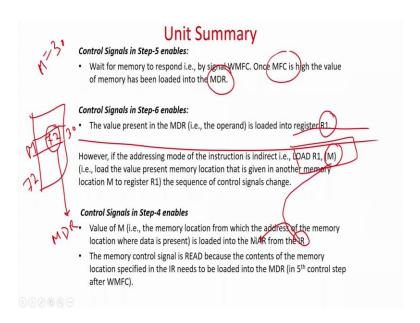
But in indirect one you have to have two memory location access. So, basically what happens in step 4, what you do basically you load the value of M, because this is your instruction you load the value of M to the from the instruction register to the memory address register. So, if you look at, this is your memory. So, let us assume that this is your memory location M say it has the value of 72, assume we can assume M = 30 say for example.
