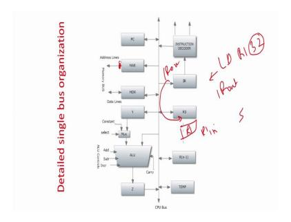
Basically already we have seen yesterday, when as I am just giving a recap because we are going to go for extending the instruction, micro instruction and the control signals based on the single bus architecture. So, if you remember we have a program counter we have memory address register. In fact, this is a unidirectional bus. So, there was a slight I mean a small error which we had taken thought of it.
