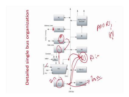
So, this 32 I am taking it from the instruction register by  $IR_{out}$  and I am putting into this memory address register. So, that the memory location value 32 whatever is in this can be com come as an operand and it will go to register  $R_1$  or wherever you want to dump that is again you want to read this value. So, this value of 32 from the IR is going to dump to memory address register.
